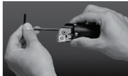
2. Tighten 3 bolts to attach the head
