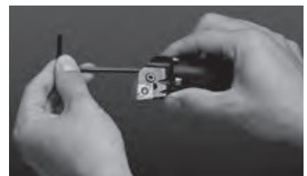
3. Tighten 3 bolts to attach the head
